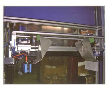
The FORMOPACK semiautomatic packing machine is designed for packing hanging clothes with a plastic film.
